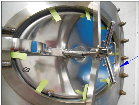
Checking door/frame bending radius and matching.
