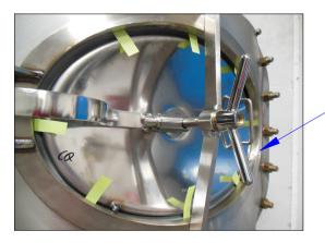
Checking door/frame bending radius and matching.
