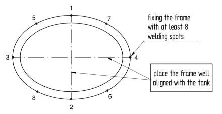
4 In order to avoid the overheating and the consequent deformation of the frame, we suggest to weld with the method TIG ( UNI ISO 287-1)
