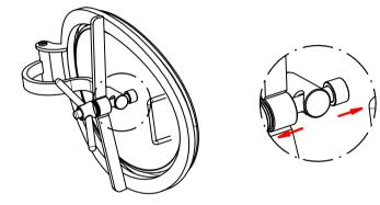
7 After welding the frame onto the tank and mounting the cover, check after tightening that the gasket adheres to the tank all along its entire perimeter.
